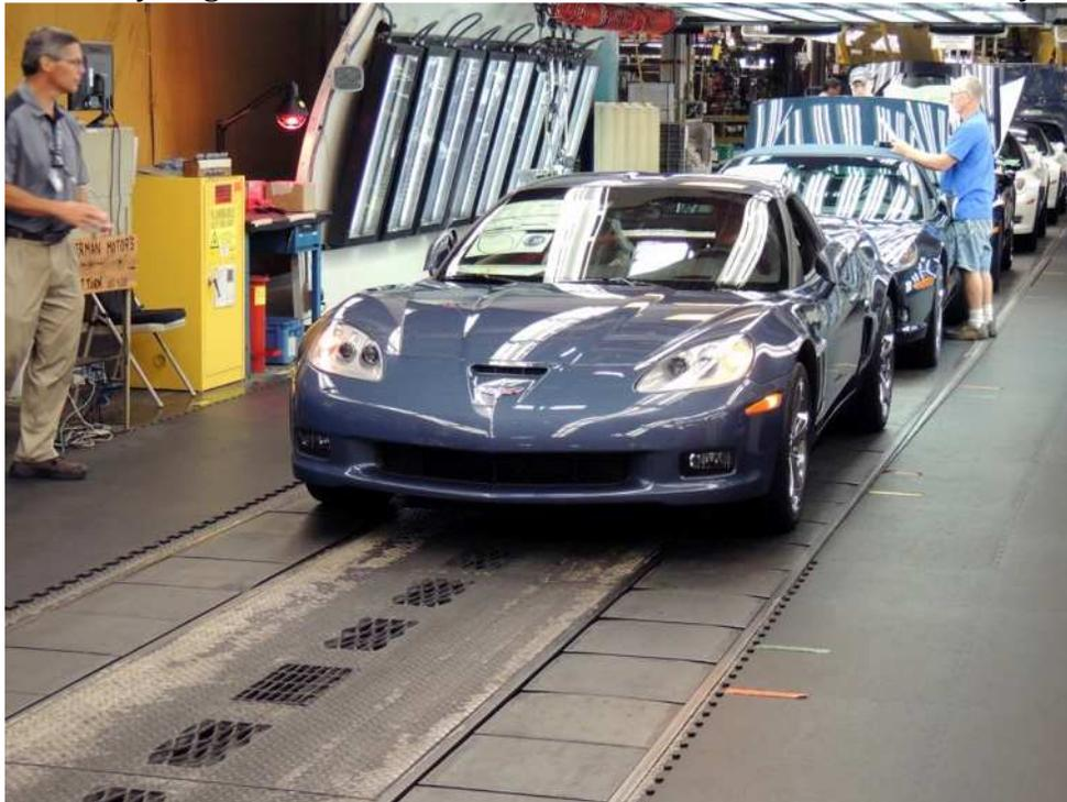
The car then went onto the alignment rack, then the dyno testing where more than 700 tests are done to verify the car systems and engine; then into the water test area, then out the door onto short test track and then the road with all the bumps and humps to check for rattles and squeaks. Fortunately our car passed all the tests.
